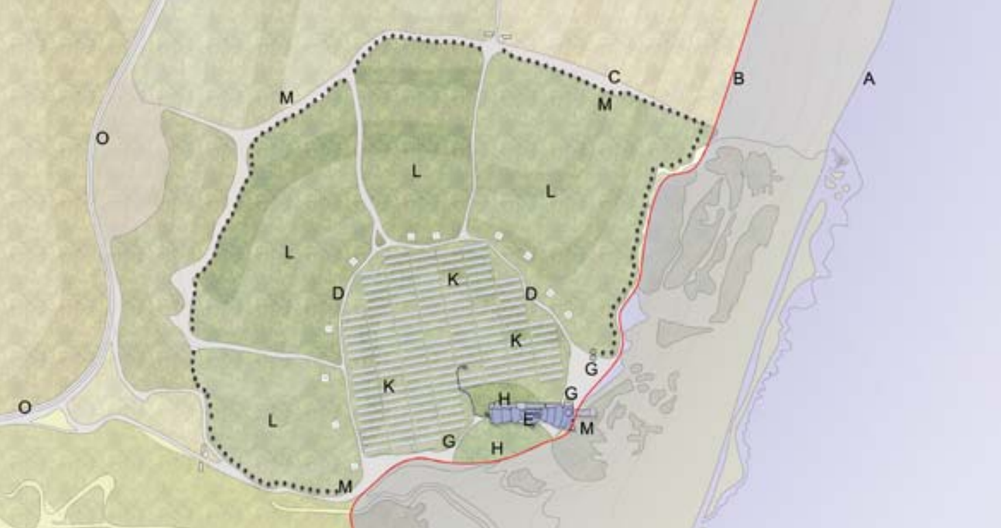
Key to Site Plan: A: The existing coast line; B: The six-metre sea rise coast line; C: The perimeter of the concept site; D: The existing tracks that will be upgraded; E: The Building for 3000 people including 'Desalination Plant', 'Archimedes Screw', 'Green House' and 'Aquaponic Tanks'; F: 'Desalination Plant' and 'Archimedes Screw'; G: Vehicle parking – mini-buses, delivery vans, water tankers and G-Wiz electric cars; H: Pleasure Gardens; J: Sewage filtration tanks; K: Five-Storey Vertical Farms; L: Trickle-irrigated Arable Land and Chicken Farms; M: Perimeter Biodiversity Margin and Solar Concentrators generating 3.5 MW of power; N: Gate Houses; O: Existing Trunk Road.
